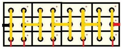
DO NOT create multiple strings of 4 series connected individual cells and put those strings in parallel, this will create unmanageable mess since individual cells in the middle of each string cannot be managed by BMS. BMS must see entire bank as 4 series connected units.
